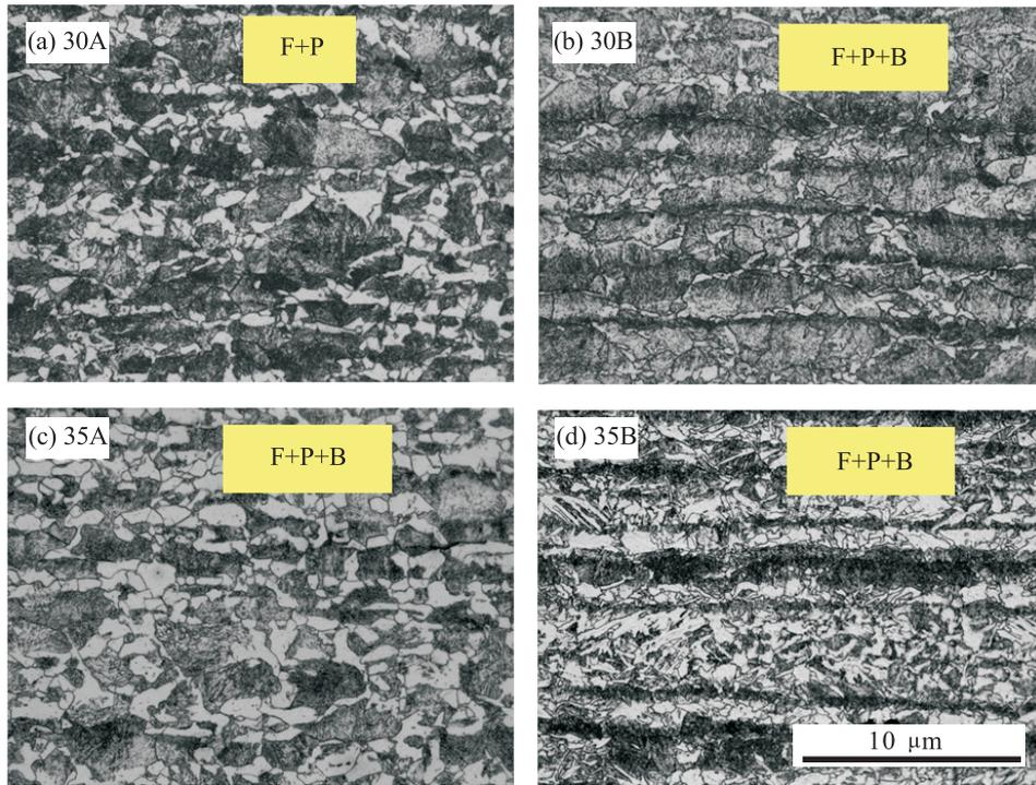
**Fig.3.** Optical microstructures of hot rolled steel alloys, (a) 30A, (b) 30B, (c) 35A and (d) 35B.
