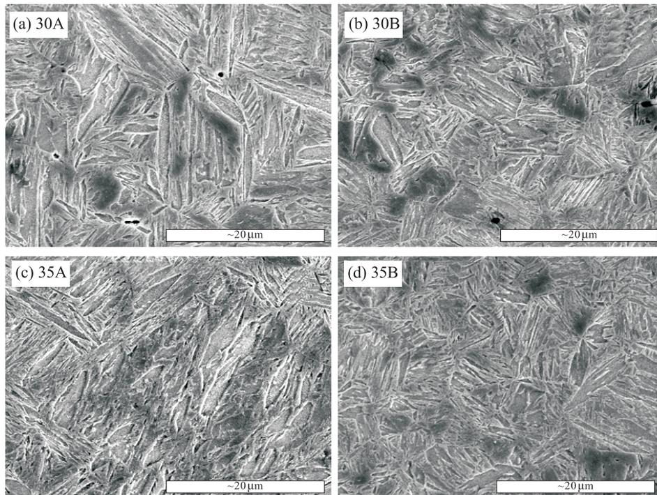
**Fig.7.** SEM microstructures of hot stamped alloys at 930°C, (a) 30A, (b) 30B, (c) 35A and (d) 35B.
