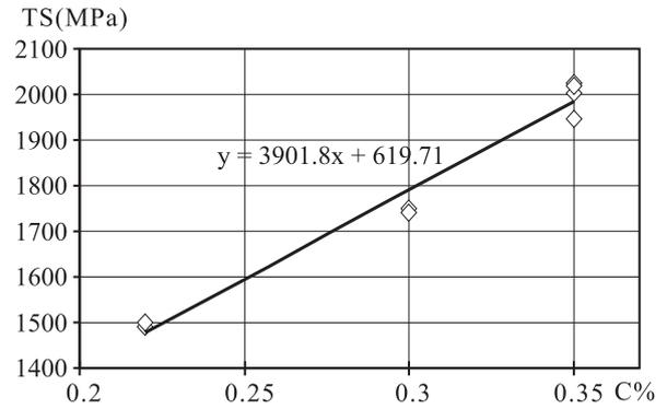
**Fig.6.** Tensile strength trend for 0.22~0.35%C MnB steels after hot stamping at 930°C.
