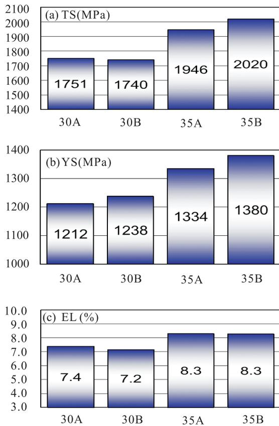
**Fig.5.** Tensile properties of cold-rolled annealed sheets after hot stamping at 930°C, (a) TS, (b) YS and (c) EL.
