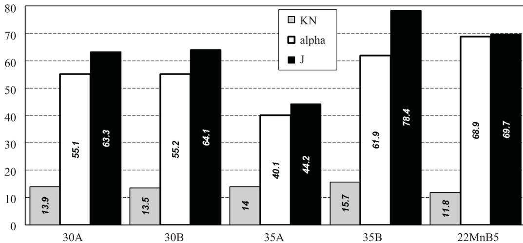
**Fig.10.** Bending properties of hot stamped alloys at 930°C.
