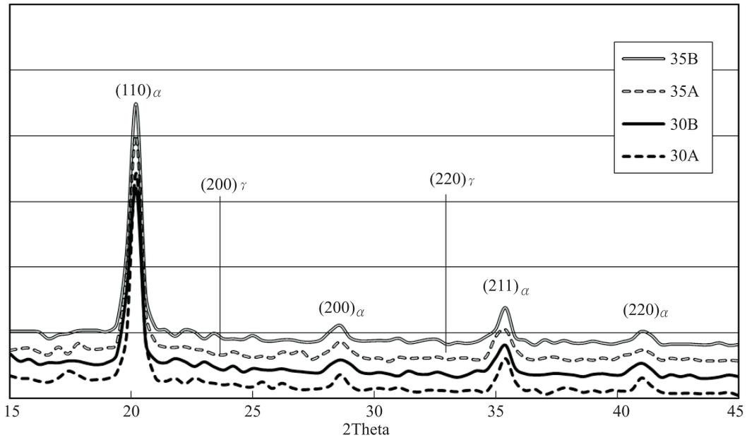
**Fig.8.** X-ray analysis of the four hot stamped alloys at 930°C.
