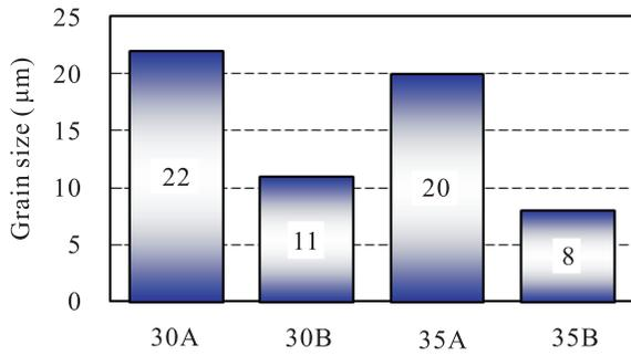
**Fig.9.** Grain size analysis of the four hot stamped alloys at 930°C.
